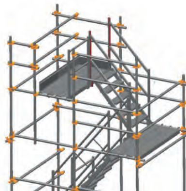
ALTERNATIVE 1M STAIR TOP LIFT
