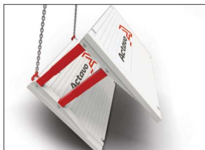
Stage 8: Stand the Drag Box upright on its cutting edges, by attaching chains to the downwards facing panel's lifting points and turn the constructed Drag Box from flat to upright.
