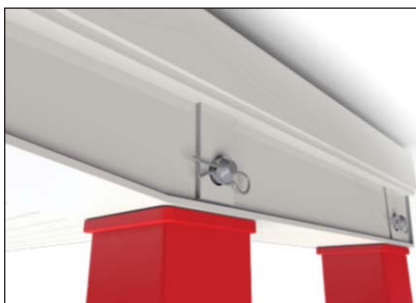
Stage 7: Lock top panel in place with clips and pins.
