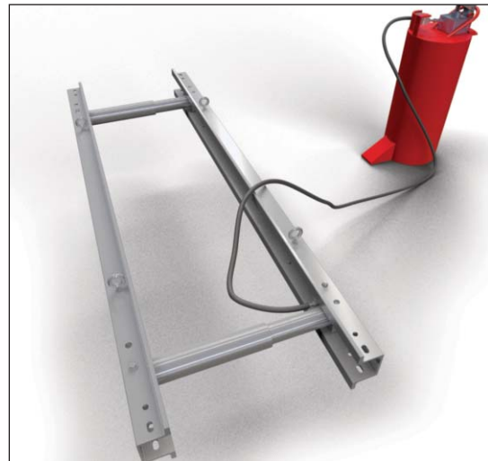
Stage 4: Pump the struts out with the Hydraulic Pump to required width.
